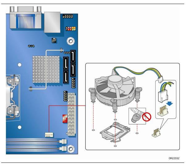
Figure 13. Connecting the Processor Fan Heat Sink Power Cable to the Processor Fan Header
